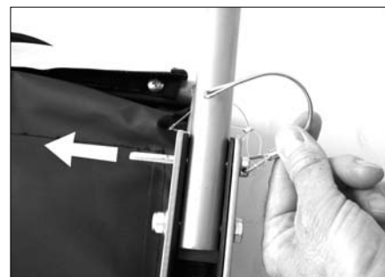
insert the securing pin through the aligned holes in the drawbar yoke and drawbar
